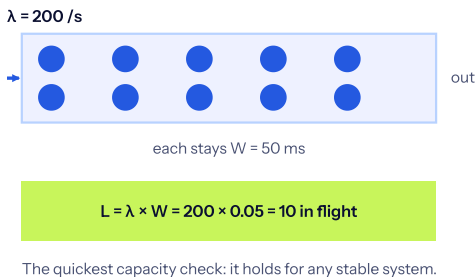
FIGURE 20 · Little's Law as a capacity check, and the arithmetic of tail latency: at 100 servers per request, 1 - 0.99^{100} \approx 63\% of requests meet at least one slow one.
